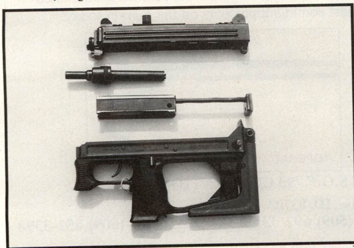
The MP-9 stripped into its four major parts component assemblies.
