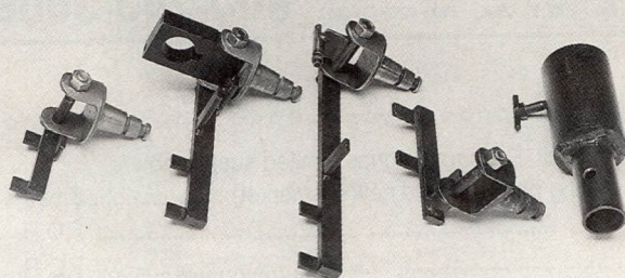
A C SHOWN W/ STANDARD BROWNING PINTLE, D W/ MODIFIED PINTLE.
