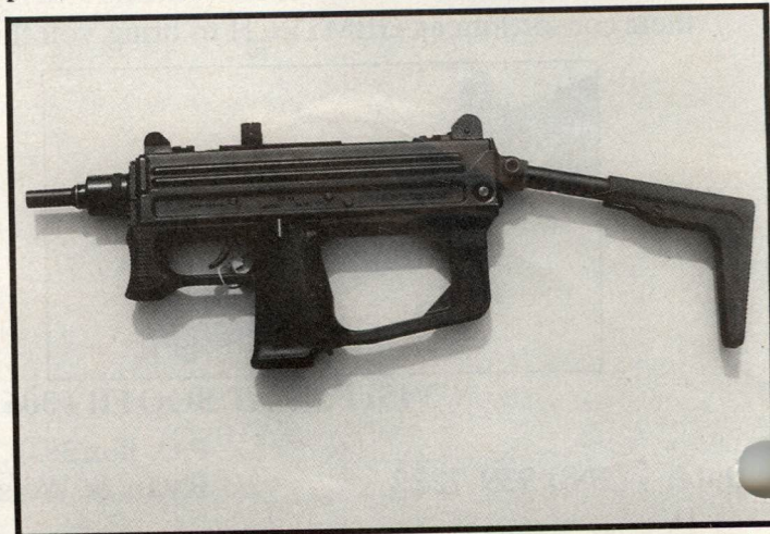
The MP-9 with stock extended still makes for a compact unit with a 21-9/10 inch overall length.
